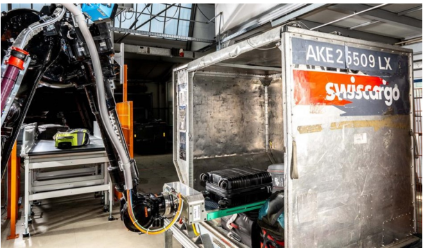
ABLE MK2 loading baggage into ULD
